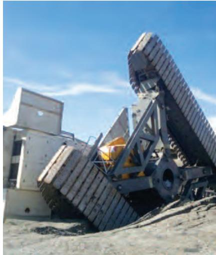
In a fatal incident at Vungtau in Vietnam, a crawler crane tipped over while lifting a load of around 315-350 tonnes in a situation where crane mats were available to spread the load and should have been used.
